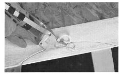
The TurboShearFC also navigates curves for window and door arcs in fiber cement siding.
